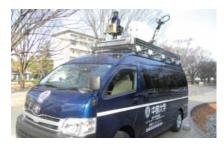
Crisis management info-collection vehicle equipped with a 360°camera, computer, plotter, satellite Internet link, and satellite mobile phone line
